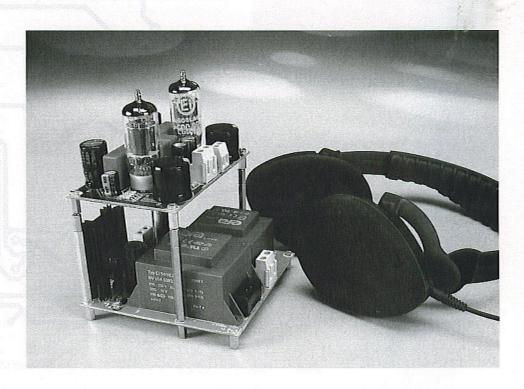
The voltage regulator requires a heat sink. Its cooling tab is connected to its middle lead, which is 0.6 V above ground potential in this circuit due to the diode.
